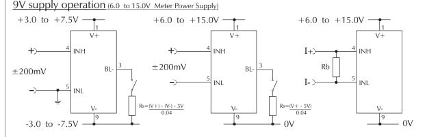
Measuring an input voltage referenced to
